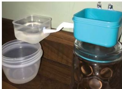
Resinktoloo - A household waste water filter, re-using sink water to flush the loo, created in response a water use brief.
